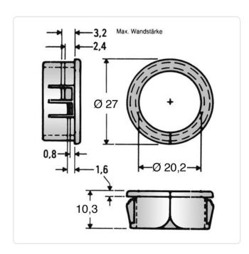
Color: Black Inner Diameter [mm]: 20.2 Material: PA 6.6 Plastic Material Group: Max. Panel Thickness [mm]: 3.2 Mounting Hole [mm]: 25.5 Outer Diameter [mm]: 27 Weight: 1.33g
