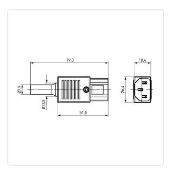
Color: Black Model: Socket Protection Code: Class 1 Wire Cross Section [mm<sup>2</sup>]: 1.0 Weight: 20g
