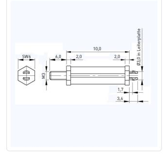
Color: Natural Flammability Class: UL94-V0 Length [mm]: 10 Material: PBT - Polybutylene Terephthalate Material Group: Plastic PCB Hole Ø [mm]: 3 PCB Thickness [mm]: 1,7 Thread Size: M3 Weight: 0.39g Conformities: Reach RoHS
