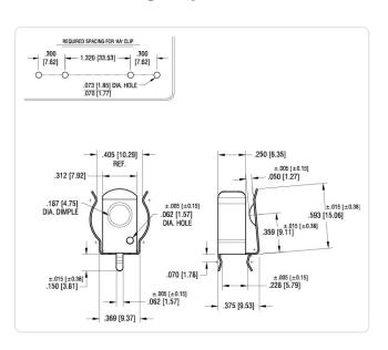
Battery Type: AA-Mignon Finish: Tin-Plated Spring Steel Material:
