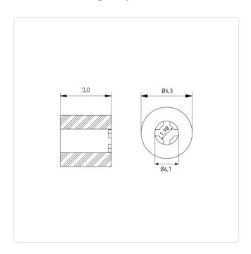
Color: Natural Flammability Class: UL94-V2 For Thread Size: M3.5 Inner Diameter [mm]: 4.1 Length [mm]: PA 6.6 Material: Material Group: Plastic
