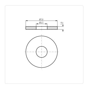
Color: Russet For Thread Size: M4 Height [mm]: Inner Diameter [mm]: 3.7
