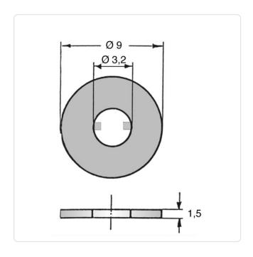
Color: Natural For Thread Size: МЗ Height [mm]: 1.5 Inner Diameter [mm]: 3.2 Material: PA 6.0 Material Group: Plastic Outer Diameter [mm]: 9
