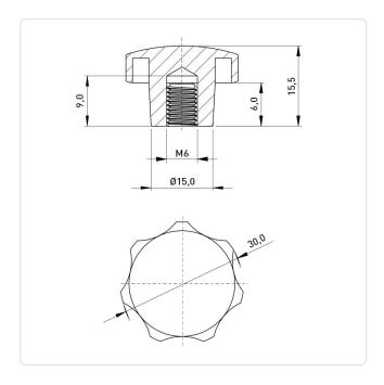
Color: Black Diameter [mm]: 30 Height [mm]: 15.5 Material: PA 6.0 Material Group: Plastic Thread Size: M6 Weight: 9.3g
