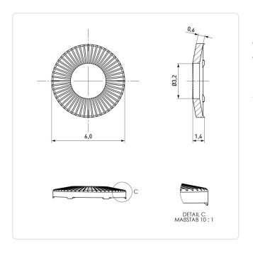
Finish: Plain For Thread Size: М3 Height [mm]: 0.6 Inner Diameter [mm]: 3.2
