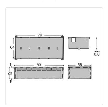
Height [mm]: 28 Length [mm]: 83 Material: Steel Material Group: Steel
