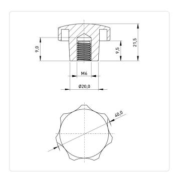
Color: Black Diameter [mm]: 40 Height [mm]: 15.5 Material: PA 6.0 Material Group: Plastic Thread Size: M6 Weight: 18.3g
