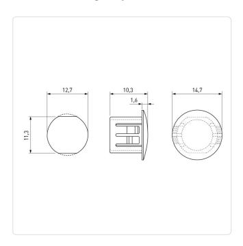
Color: Black UL94-V2 Flammability Class: Head Diameter [mm]: 14.7 Head Height [mm]: 11.3 Material: PA 6.6 Material Group: Plastic Snap-In Model: Mounting Hole [mm]: 12.7
