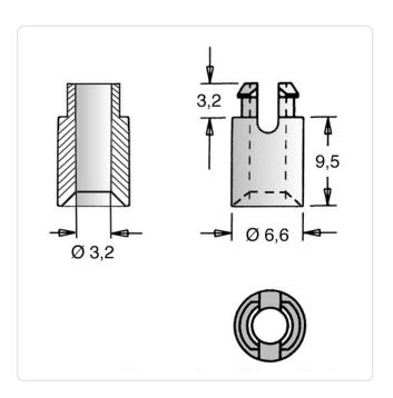
Color: Natural Flammability Class: UL94-V2 For Thread Size: М3 Inner Diameter [mm]: 3.2 Length [mm]: 9.5 Material: PA 6.6 Material Group: Plastic Mounting Hole [mm]: 4.8 Outer Diameter [mm]: 6.6 Weight: 0.27g
