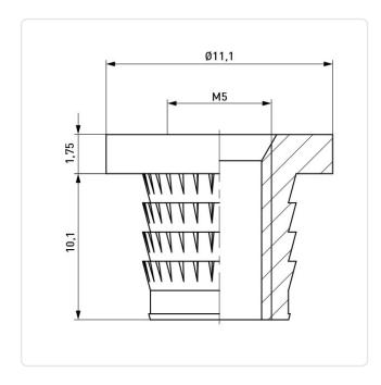
Finish: Plain Head Diameter [mm]: 11.1 Length [mm]: 10.1 Material: Brass Material Group: **Brass** Minimum Edge Distance [mm]: 2.9 Panel Hole Ø [mm]: 6.5 Thread Size: M5 Weight: 2.4g
