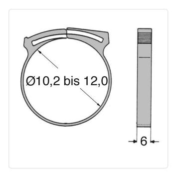
Color: Black Flammability Class: UL94-V2 Material: PA 6.6 Material Group: Plastic Panel Thickness Range [mm]: 10,2-12,0 1.8 Thickness [mm]:
