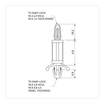
Color: Natural Flammability Class: UL94-V2 Length [mm]: 4.8 PA 6.6 Material: PCB Hole Ø [mm]: 4 PCB Thickness [mm]: 1,6 Panel Hole Ø [mm]: 4.8 Panel Thickness [mm]: 0,8-2,0 Weight: 0.36g
