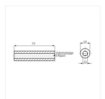
Color: Black Flammability Class: UL94-V2 For Thread Size: М3 Inner Diameter [mm]: 3.4 Length [mm]: 2 Material: PA 6.6
