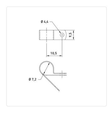
Bundle Diameter [mm]: 7,2 Color: Natural Distance Middle/Middle [mm]: 10.5 UL94-V2 Flammability Class: Material: PA 6.6 Material Group: Plastic Mounting Hole [mm]: 4.4 Thickness [mm]: 1.4 Width [mm]: 9.5
