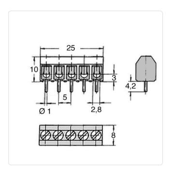
Finish: Tin-Plated Flammability Class: UL94-V0 Grid [mm]: 5.0 Material: PA 6.0 Panel Thickness Range [mm]: 1,5
