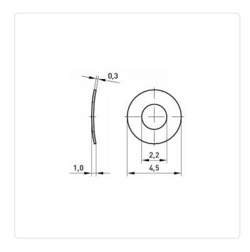
DIN/ISO: DIN137A Finish: Plain For Thread Size: M2 0.3 Height [mm]: Inner Diameter [mm]: 2.2
