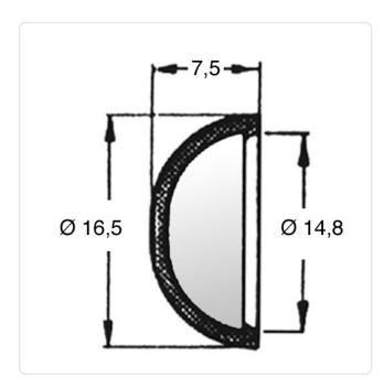
Color: Black Head Height [mm]: 7.5 Inner Diameter [mm]: 14.8 PA 6.0 Material: Material Group: **Plastic**
