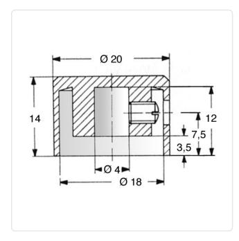
14 Height [mm]: Inner Diameter [mm]: 4
