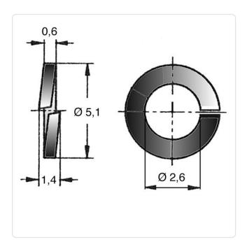
DIN/ISO: DIN127B Finish: Plain For Thread Size: M2.5 0.6 Height [mm]:
