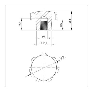
Color: Black Diameter [mm]: 50 Height [mm]: 21.5 Material: PA 6.0 Material Group: Plastic Thread Size: M6 Weight: 21g
