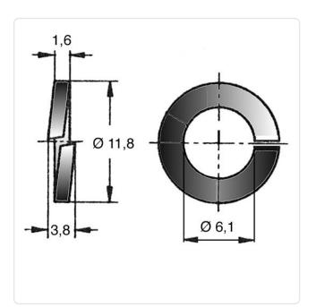
DIN/ISO: DIN127B Finish: Plain For Thread Size: M6 1.6 Height [mm]:
