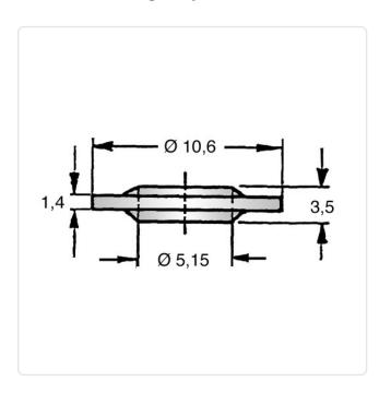
For Thread Size: M5 3.5 Height [mm]: Inner Diameter [mm]: 5.15 Material: PA 6.0 Material Group: **Plastic** Outer Diameter [mm]: 10.6 Weight: 0.12g
