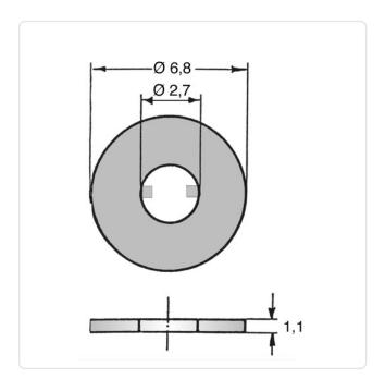
Color: Natural For Thread Size: M2.5 Height [mm]: 1.1 Inner Diameter [mm]: 2.7 Material: PA 6.0 Material Group: Plastic Outer Diameter [mm]: 6.8 Weight: 0.04g
