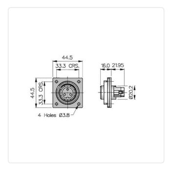
Amperage [A]: 10 Color: Black Protection Code: IP68 Weight: 33g Conformities:
