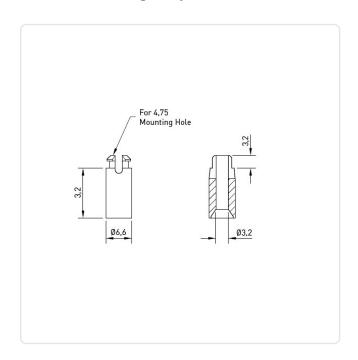
Color: Natural Flammability Class: UL94-V2 For Thread Size: М3 Inner Diameter [mm]: 3.3 Length [mm]: 3.2 Material: PA 6.6 Material Group: Plastic Mounting Hole [mm]: 4.8 Outer Diameter [mm]: 6.6
