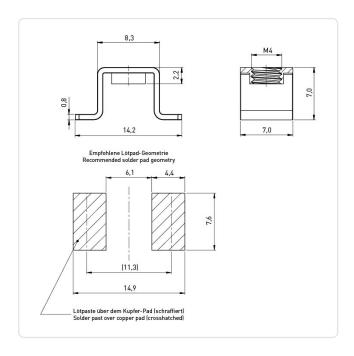
Finish: Plain Grid [mm]: 7.0 Material: **Brass** Material Group: Brass Thread Size: M4 Weight: 0.25g Conformities:
