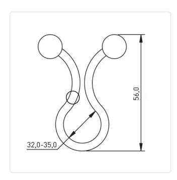
Bundle Diameter [mm]: 30,0-40,0 Color: Natural Flammability Class: UL94-V2 Material: PA 6.6 Material Group: Plastic Weight:
