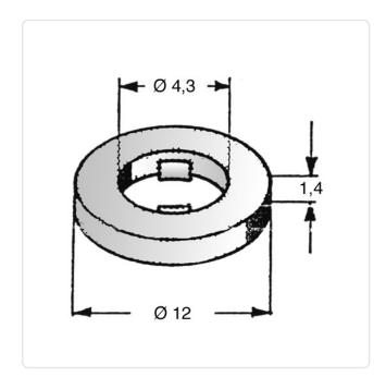
Color: Black For Thread Size: M4 Height [mm]: 1.5 Inner Diameter [mm]: 4.3
