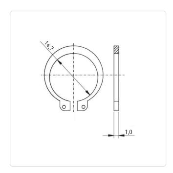
DIN/ISO: **DIN471** Finish: Plain Height [mm]: Inner Diameter [mm]: 16
