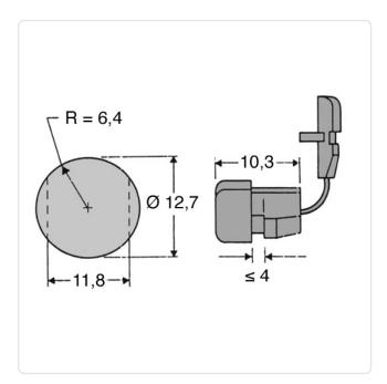
Cable diameter [mm]: Ø 3,8-7,6 Color: Black Material: PA 6.6 Material Group: Plastic Mounting Hole [mm]: 12.7 Panel Thickness Range [mm]: 3.8x7.6 Panel Thickness [mm]:
