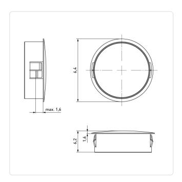
Color: White Flammability Class: UL94-V2 Head Diameter [mm]: 6.4 Head Height [mm]: 1.6 PA 6.6 Material: Material Group: Plastic Model: Snap-In Mounting Hole [mm]: 4.8
