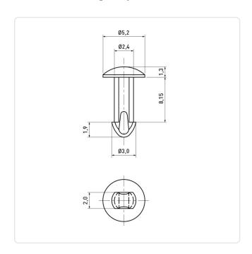
Color: Red Flammability Class: UL94-V2 Head Diameter [mm]: 5.2 Material: PA 6.6 Material Group: **Plastic** Mounting Hole [mm]: 2.5 Weight:
