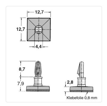
Color: Natural Flammability Class: UL94-V2 Length [mm]: 7.9 Material: PA 6.6 PCB Hole Ø [mm]: 3.2 PCB Thickness [mm]: 1,6 Weight:
