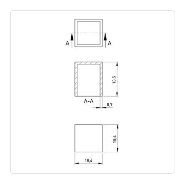
Color: Black Flammability Class: UL94-V2 Height [mm]: 13.5 18.4 Length [mm]: PA 6.6 Material: Material Group: Plastic
