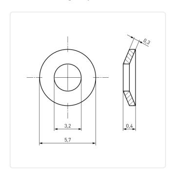
Finish: Plain For Thread Size: М3 0.3 Height [mm]: Inner Diameter [mm]: 3.2
