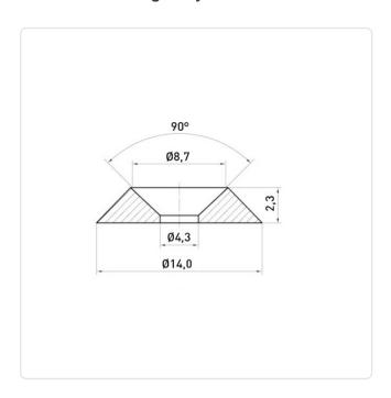
Finish: Plain For Thread Size: M4 Height [mm]: 2.3 Inner Diameter [mm]: 4.3
