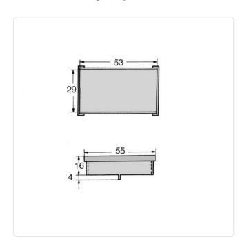
Height [mm]: 16 Length [mm]: 54 Material: Steel Material Group: Steel
