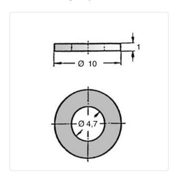
Color: Russet For Thread Size: M5 Height [mm]: Inner Diameter [mm]: 4.7
