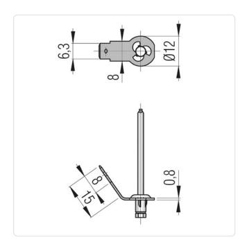
Finish: Plain Material: **Brass Brass** Material Group: Mounting Hole [mm]: 5.2 Panel Thickness [mm]: 0,6-2,0 Plug-In Length [mm]: 7.8 Size [mm]: 6.3x0.8 Tabs:
