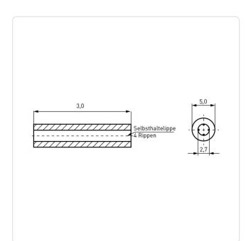
Color: Black Flammability Class: UL94-V2 For Thread Size: M2.5 Inner Diameter [mm]: 2.7 Length [mm]: Material: PA 6.6
