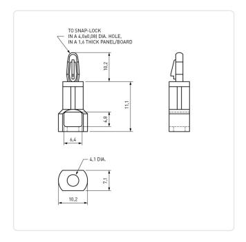
Color: Natural UL94-V2 Flammability Class: 11.1 Length [mm]: PA 6.6 Material: Material Group: **Plastic** PCB Hole Ø [mm]: PCB Thickness [mm]: 1,6 Panel Hole Ø [mm]: 4.1 Weight: 0.51g
