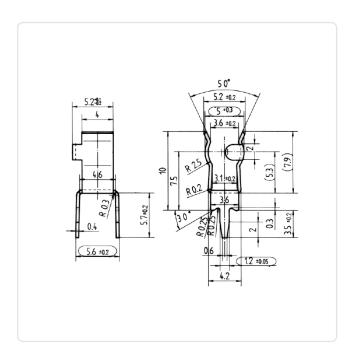
Fuse Size [mm]: 5.0x20.0 Material: **Brass** Material Group: **Brass** Model: Clip Holder
