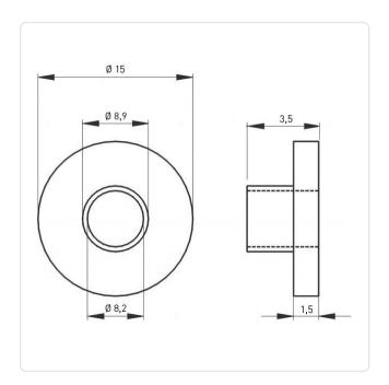
Color: Natural Flammability Class: UL94-V2 Height [mm]: 3.5 Inner Diameter [mm]: 8.2 Lug Diameter [mm]: 8.9 Material: PA 6.0 Material Group: Plastic
