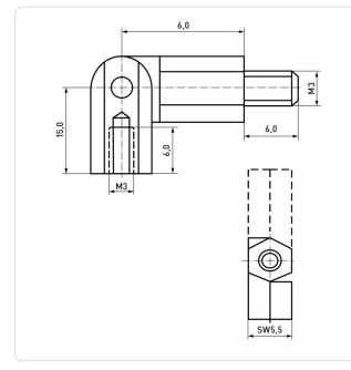
Finish: Nickel-Plated, 3 µm, E1E Leg Length 1 [mm]: 6 Leg Length 2 [mm]: 15 21 Length [mm]: Material: Brass Material Group: Brass Model: Male/Female M3 Thread 1 Size: Thread 2 Size: М3 Weight: 4.06g Conformities: Reach RoHS SVHC
