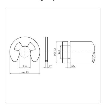
DIN/ISO: **DIN6799** Finish: Plain Height [mm]: 0.7 Inner Diameter [mm]: 4
