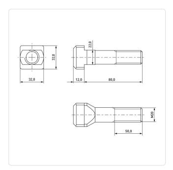
DIN/ISO: **DIN787** Finish: Plain Head Height [mm]: 12
